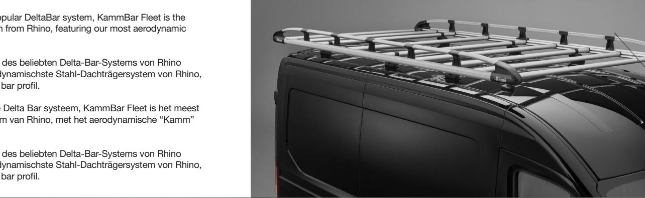
The successor to the incredibly popular DeltaBar system, KammBar Fleet is the most durable steel roof bar system from Rhino, featuring our most aerodynamic "Kamm" bar profile.
