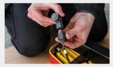
Click each sensor into the wiring loom provided with the step (note: this is shown without the step fitted here for illustrative purposes).
