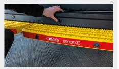
Use panel blanking plug to fill space where the sensors previously were located on the vehicle.
