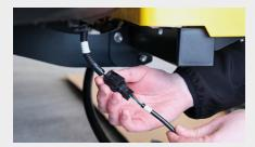
Connect the other end of the sensor into the van's wiring harness and cable tie all vehicle wiring securely back in place.
