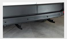
Fit the outriggers to the vehicle's under-chassis mounting points and fit the step to the other end.
