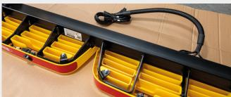
Making alterations to introduce an external step with parking detection technology has previously been a time-consuming process, often requiring specialist knowledge, complicated rewiring and of course, added expenditure. Connect+ neatly solves this problem by integrating each OEM sensor into the step via a simple 'plug and play' cable.
