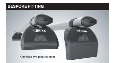
Available in two, three and four bar configurations, the KammBar Fleet comes complete with a fitting kit that includes bespoke pads and spacers, tailored to the mounting points of every vehicle.
