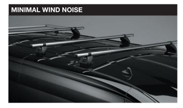
The KammBar Fleet's aerodynamic shape almost entirely eliminates wind noise.
