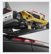
Rubber inserts on the brace bar, reducing rattling noise while in transit \*A padlock can be added\*
