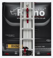
2 belts top and bottom to hold ladder tightly in place and eliminate rattling
