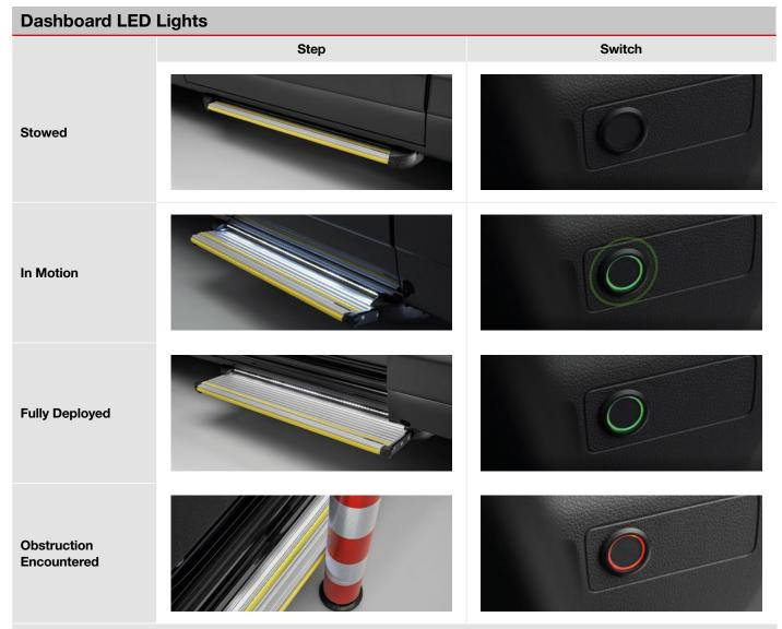
The step is configured to deploy automatically when the vehicle door is opened and to stow when the door is closed (note: the circular dashboard switch needs to be pressed to power the step).
