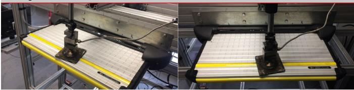
The Glide Step has undergone a rigorous series of tests to ensure safety, reliability and premium performance. This includes cycle load testing, increasing weights in both central and off-centre positions for tens of thousands of cycles.
